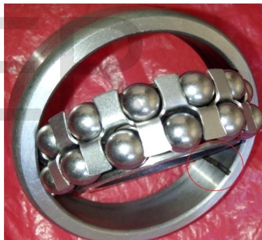
Fig. 3 Fault created on outer race
